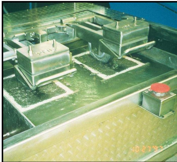
**Figure 1. Hamburg Wheel-Tracking Device**
